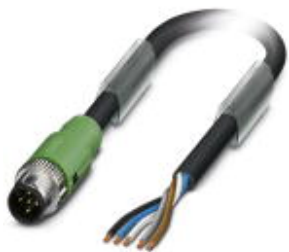
Sensor/actuator cable, 5-position, PUR, black-gray RAL 7021, Plug straight M12 SPEEDCON, A-coded, on free cable end, cable length: 2 m
